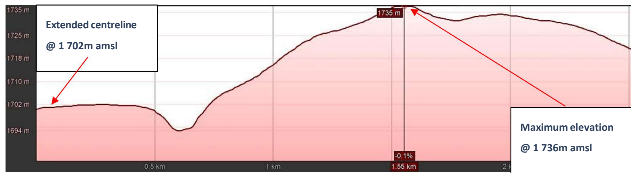
Figure 7: Elevation Profile from Extended Runway Centreline along western boundary of Bokamoso Site
